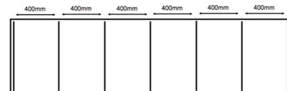
**Step 8: APPLYING ADHESIVE** - Apply a 6mm bead of high strength, water resistant construction adhesive - recommended to use the Dow Corning 680 Silicone (Lincoln Product Code: 2-152-831 white or 2-152-830 translucent) in a wavy pattern between each tape strip, as shown.
